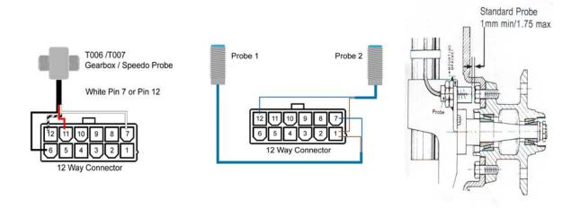
Bolt head pickup must be flat steel and should cover a minimum 80% of the probe head
